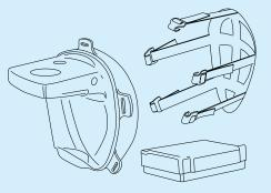
**TikiUSER** Mask, harness and a filter in a soft bag. Mask sizes medium or large.
