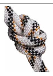
ThermoCore technology consists in consolidating the sheath and the core of the rope by hot-melt process to suppress "the socket" sliding effect. This is achieved with a specific treatment of the rope under tension at  $150^{\circ}$  C.
